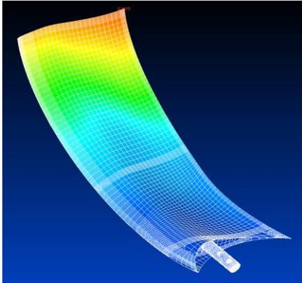
Detailed modal analysis is carried out to determine the natural frequencies of the various components of the wind turbine. Frequency response and transient response analyses are also carried out to determine critical deflections under forced oscillations caused by changing wind direction. Interference between various components of the wind turbine is analyzed and the structure is designed as per
