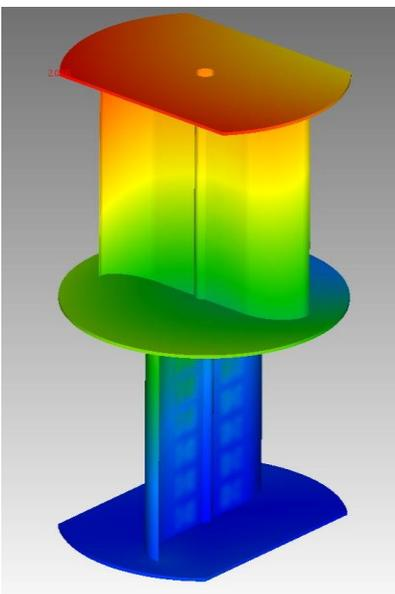
non-linear cases are analyzed. The structure can be made out of steel, aluminum, glass fiber and/or carbon fiber or any combination thereof. A unique method has been developed by DARcorporation engineers to analyze the harmonic behavior of wind turbines. Unwanted vibrations are detected and designed out of the system.
